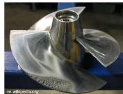
Damage on propeller blades
