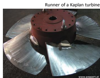
Runner of a Kaplan turbine
