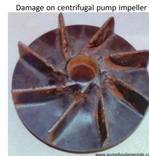
Damage on centrifugal pump impeller
