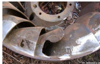
Damage on Francis turbine blades
